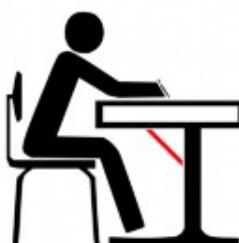
The Under Desk Heater (UDH) is designed to be mounted under a desk at a 45 degree angle using 4 mounting brackets located on the sides of the panel.
